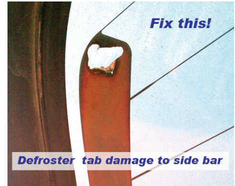
Badly damaged defroster occurred when the tab pulled some of the defroster material away from the glass.
