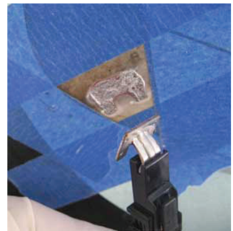
Mask off damaged area
