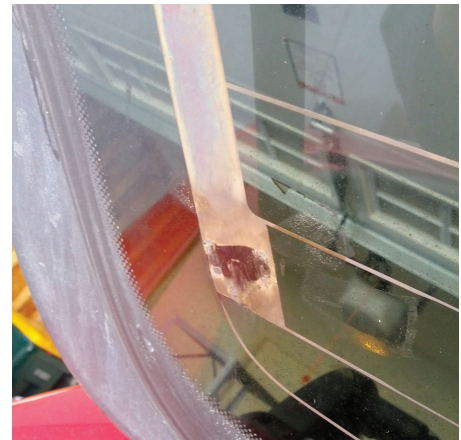
More defroster damage
