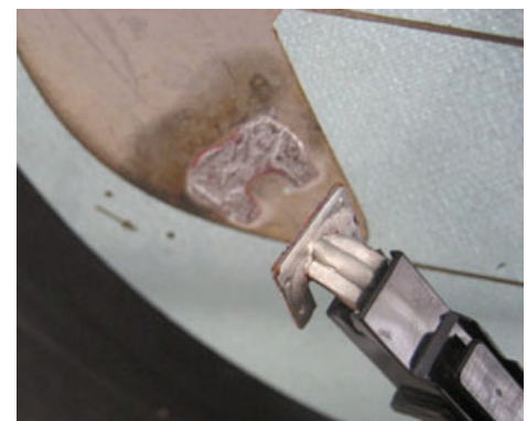
Damaged defroster pad
