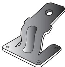
Applying heat with a hair dryer or heat gun while applying force with pliers can be effective. Care must be given not to break the glass when removing the tab.
