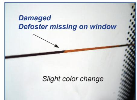
Second, the defroster conductor has a physical presence on the glass so there should be a tiny bump on the glass surface that can be felt when moving your finger across the grid line. If everything is perfectly smooth then it's a good bet the defroster is missing.
