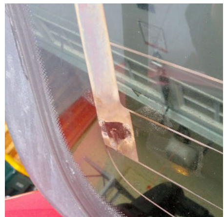
More defroster damage
