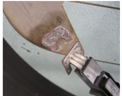
Damaged defroster pad
