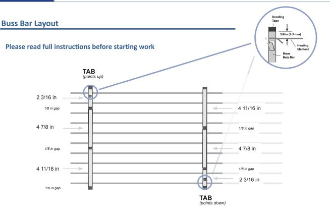
The gap between the buss bars is 1/8 in (32 mm) and is critical.
