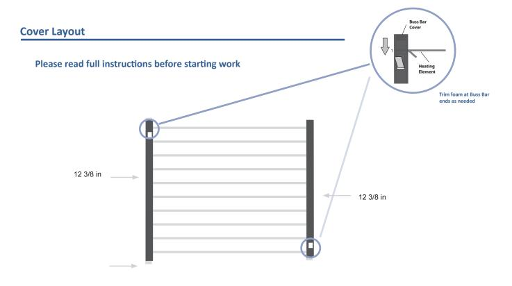
Apply the cover only after the elements have been connected over the buss bar. Press cover down firmly to seat adhesive.
