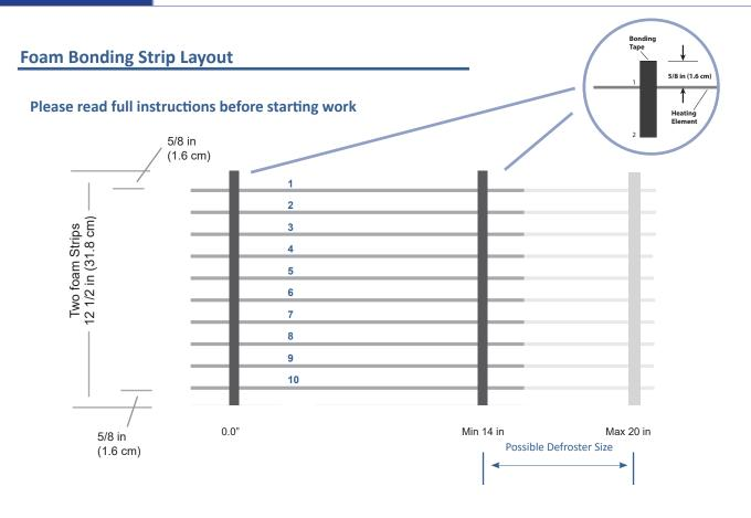
Do not stretch the foam bonding strips
