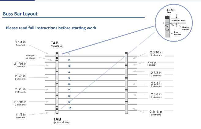
The layout, number of elements per buss bar and the 1/8 in (32 mm) gap between are CRITICAL.
