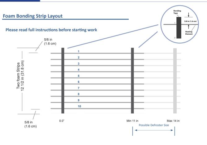
Do not stretch the foam bonding strips
