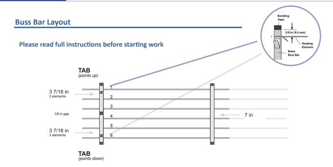
The gap between the buss bars is 1/8 in (32 mm) is critical.
