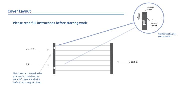
Apply the cover only after the elements have been connected over the buss bar.
