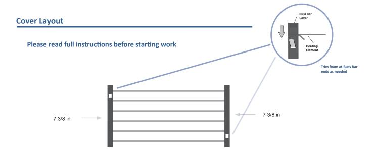
Apply the cover only after the elements have been connected over the buss bar. Press cover down firmly to seat adhesive.
