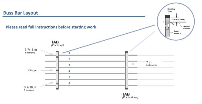
The layout, number of elements per buss bar and the 1/8 in (32 mm) gap between are CRITICAL.
