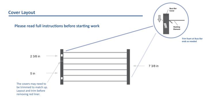
Apply the cover only after the elements have been connected over the buss bar. Press cover down firmly to seat adhesive.
