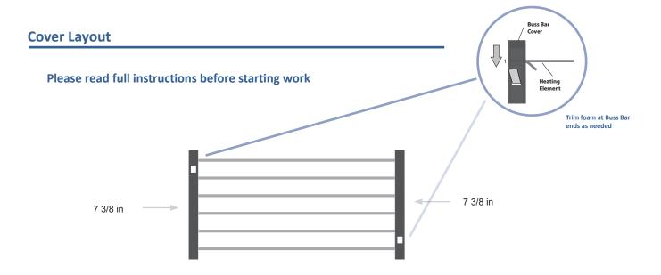
Apply the cover only after the elements have been connected over the buss bar. Press cover down firmly to seat adhesive.
