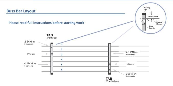
The layout, number of elements per buss bar and the 1/8 in (32 mm) gap between are CRITICAL.
