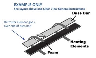
Defroster side buss bars go on top of foam as shown above. Make a good metal to metal contact.
