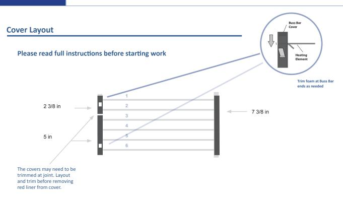
Apply the cover only after the elements have been connected over the buss bar.
