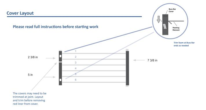
Apply the cover only after the elements have been connected over the buss bar.
